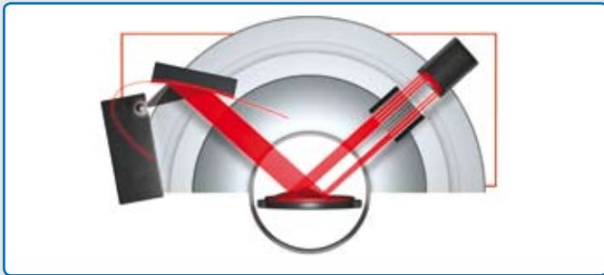
Fig. 4a: Phase ID Mirror beam path - XRPD on irregularly shaped sample.
