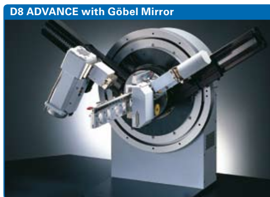
Fig. 1: D8 ADVANCE with Göbel Mirror and Flip-Stick sample changer.
