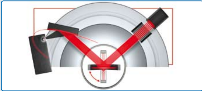
Fig. 2a: Multipurpose Göbel Mirror beam path – XRPD in reflection and transmission on the same sample or in the same sample batch.
