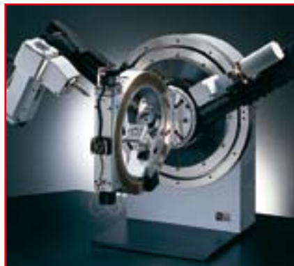
Fig. 2. Closed circle Eulerian cradle on vertical D8 goniometer for texture investigations
