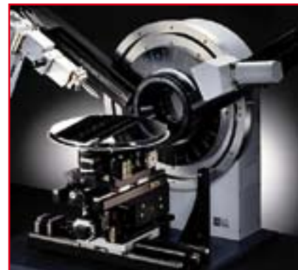
Fig. 4. UMC 300 stage for thin film studies
