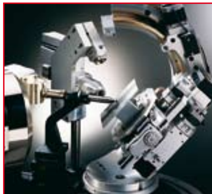
Fig. 3. 1/4-circle Eulerian cradle for residual stress investigations
