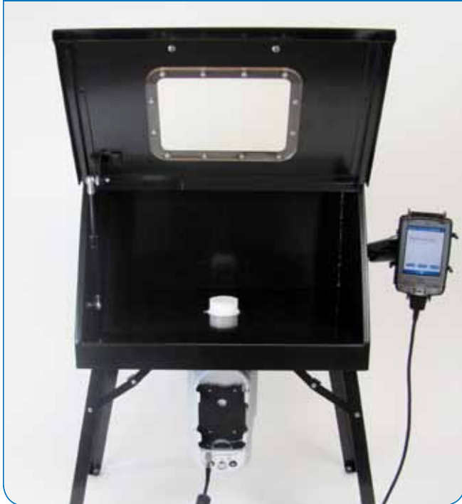
S1 TURBO SD with bench-top stand and sample cup
