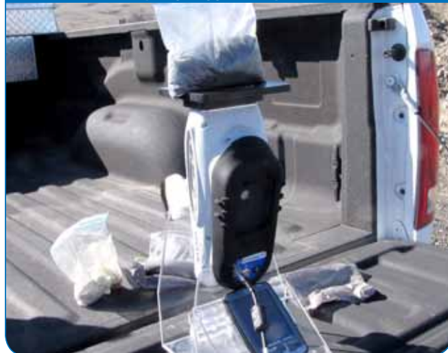
S1 TURBO SD analyzing bagged samples
