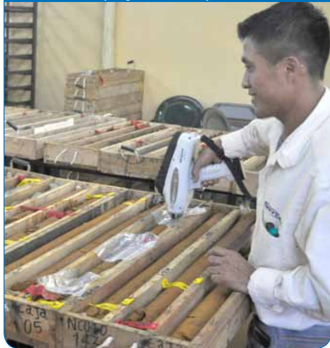
S1 TURBO SD analyzing drill core samples
